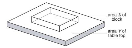
The area of the block in contact with the table is X and the area of the table top is Y.
